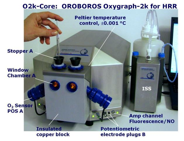
The O2k-Core (Series G, compare Series H) is the experimental system complete for basic high-resolution respirometry (HRR), including the O2k-Main Unit with stainless steel housing, O2k-Assembly Kit, two OroboPOS (oxygen sensors), and OroboPOS-Service Kit, DatLab software (DatLab), ISS-Integrated Suction System and O2k-Titration Set. The O2k-Core supports all add-on O2k-Modules.
