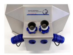
1. Dry the chamber. Remove all liquid droplets from the glass chamber. Place a dry PVDF stirrer bar into each chamber.
