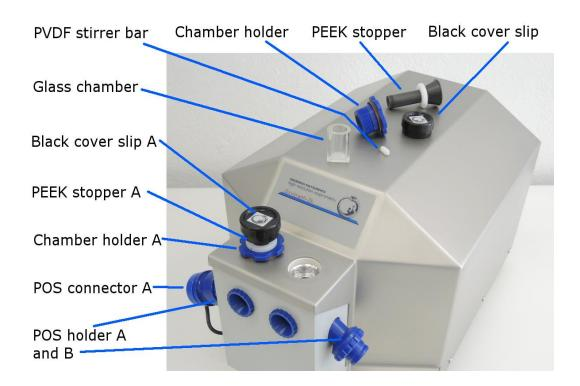
Unscrew the blue chamber holders from the O2k housing. Remove the POS connectors from the POS holders by pressing the sleeve downwards against the bottom plate of the POS connector. Unplug the cable.
