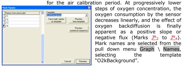
steps of oxygen concentration, the oxygen consumption by the sensor decreases linearly, and the effect of backdiffusion oxygen is apparent as a positive slope or negative flux (Marks  $J_{2}^{\circ}$  to  $J_{4}^{\circ}$ ). Mark names are selected from the pull down menu Graph \ Names, selecting the template "O2kBackground".
