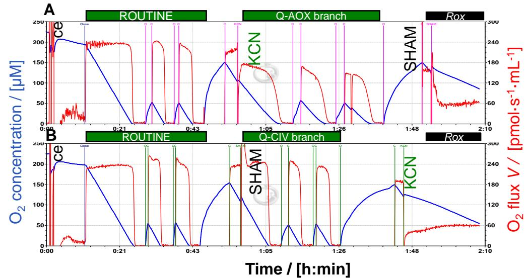
O2k traces of O<sub>2</sub> kinetics with repeated aerobic-anoxic transitions and re-oxygenations. (A) SUIT-022\_02\_ce\_D051 protocol. (B) SUIT-023\_02\_ce\_D053 protocol. [www.bioblast.at](http://www.bioblast.at)
